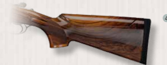
'Parcours' stock (Fig. 4) adjustable, vertically 14 mm, horizontally 10 mm optional non-adjustable stocks available Length: 365 mm, Drop: 42 mm / 50 mm Stock finish: Oil
